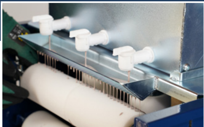
Practical nozzles with tap opening for adjusting the amount of colour to impregnate the sponge rollers*.
