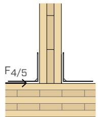
The F<sub>4</sub>, F<sub>5</sub>, F<sub>4/5</sub> values in the table are valid for the acting stress calculation eccentricity e=0 (timber elements prevented from rotating).
