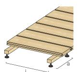
The number of supports per  $m^2$  is to be assessed according to the load magnitude and the joist spacing.
