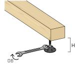
Adjust the height of the support from the bottom using a 10 mm SW wrench.
