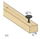
Screw the support into the bushing and turn the joist.
