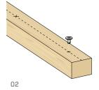
The depth of the pre-drill depends on the assembly height R and must be at least 16 mm (bushing size).
