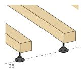
Place the joist on the substrate, parallel to the one previously laid.
