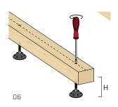
Adjust the height of the support from above using a flat screwdriver.
