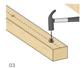
Use a hammer to insert the bushing.
