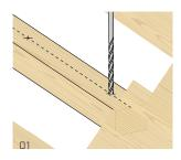
Trace the joist midline, indicating the position of the holes and then pre-drill a 10 mm diameter hole.
