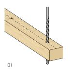
Trace the joist midline, indicating the position of the holes and then pre-drill a 10 mm diameter through hole.
