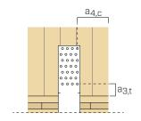
WHT PLATE T plates are designed for different floor thickness values including resilient acoustic profile. The positioning notches, as an assembly aid, indicate the maximum permitted distance (D) between the CLT wall panels in compliance with the minimum distances for HBS PLATE Ø8 mm screws. This distance includes the space required for the acoustic profile housing ( $s_{acoustic}$ ).
